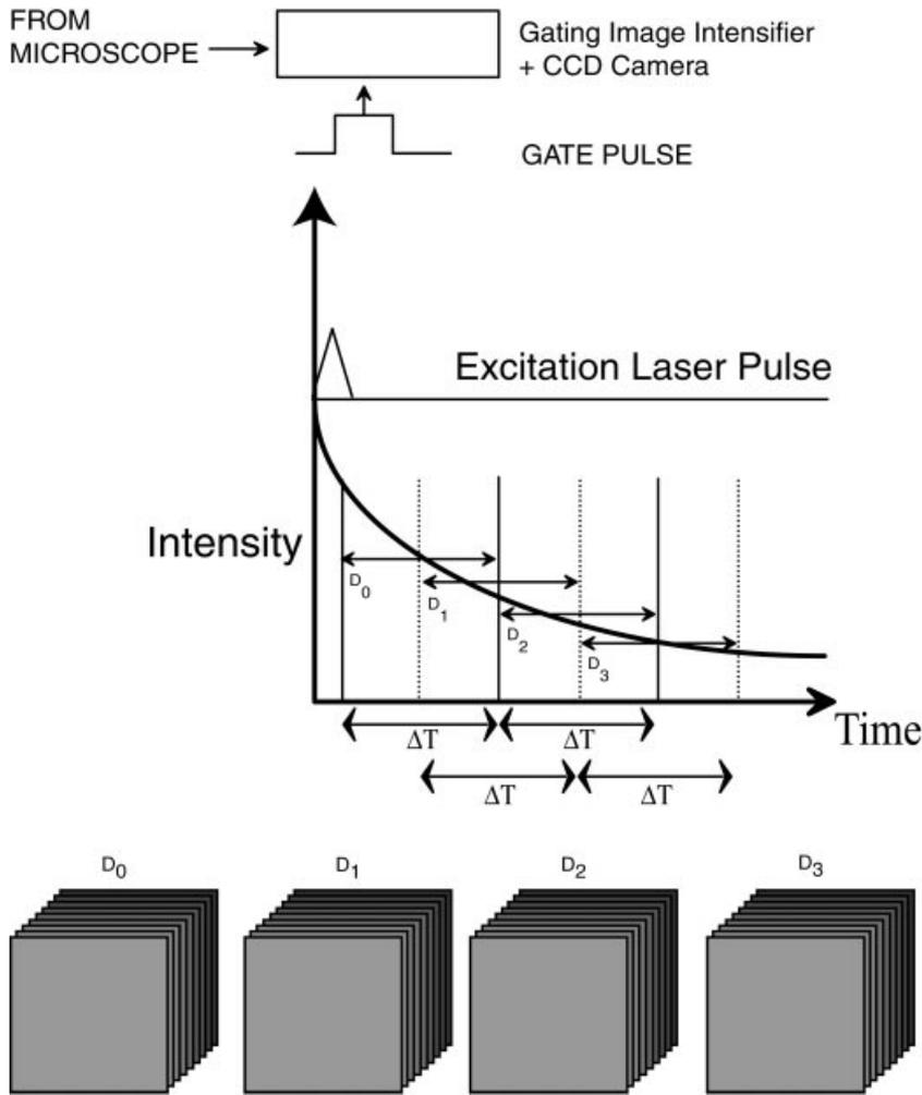
Fig. 2. Schematic illustration for the acquisition of time-resolved FLIM images. After laser pulse excitation the reference pulse from the laser was used as a trigger pulse to gate the camera. The first gate image ( $D_0$ ) was acquired with gate window (or exposure time) of  $\Delta T$ . This signal was accumulated for a certain duration of time  $t$ . Likewise, other ( $D_1, D_2$  and  $D_3$ ) gated images were acquired.
