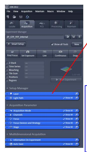
Turned on laser through the software by selecting "ON"
