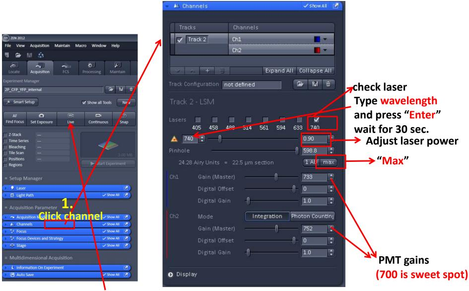
2. Click "Live" after selecting the laser, pinhole, channels. In live mode, adjust power, gain etc.
