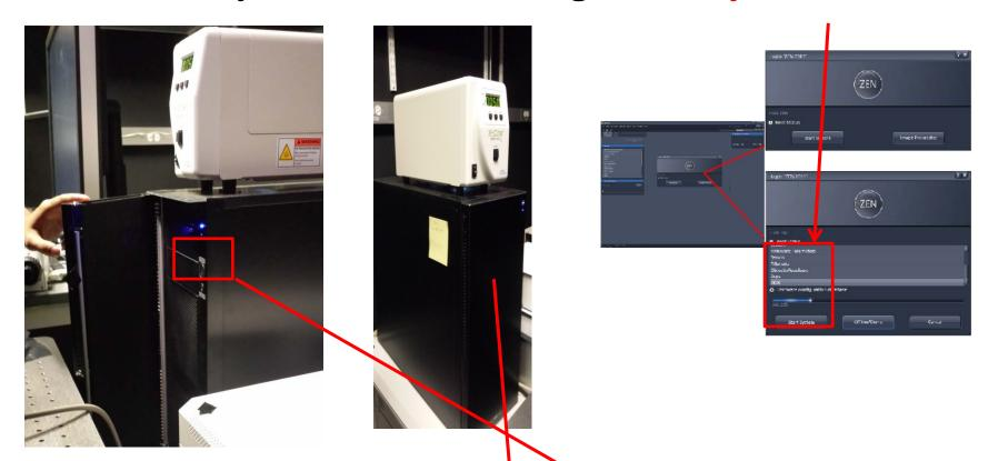
If you see any error message such as "Software stops working" then close the software and "log off". After that reboot your machine. Press the big button, wait for 5 minutes and restart the Zen software.
