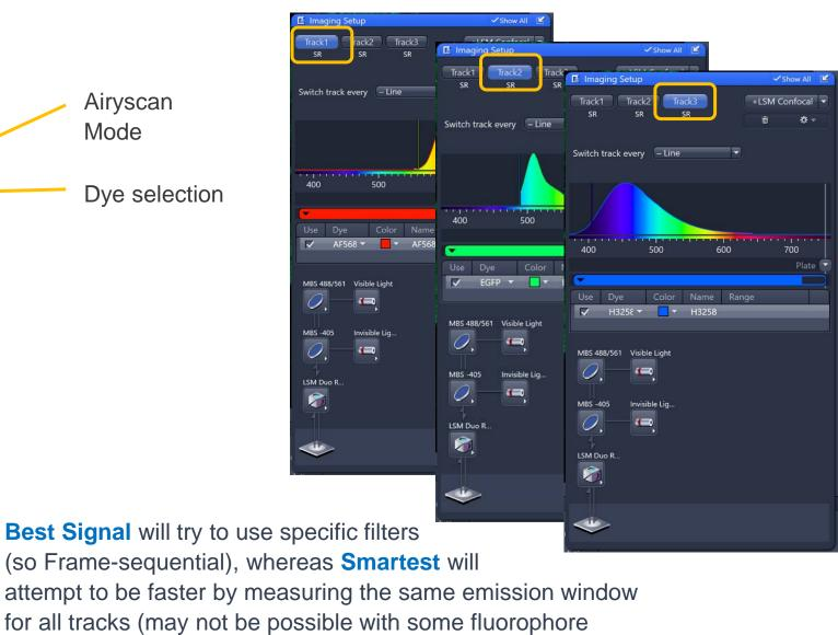
**SR Mode:** (1) Maximum gain in resolution and SNR; Pinhole default 0.2 AU; Total detection area 1.25 AU
