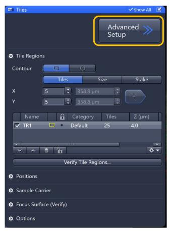
Tick tiles in experiment window and expand the **Tiles** tab. Add **Tile Regions** using the Advanced Set up. **Live** in a separate container may get used to set the best focus position.
