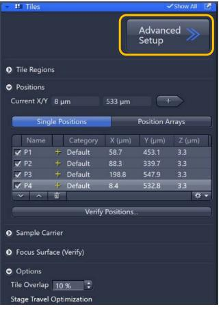
Tick tiles in experiment window and expand the **Tiles** tab. Add **Positions** using the Advanced Set up: this can also be used to map carrier templates.
