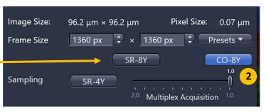
Maximum Scan Speed (SR-4Y mode: 25 fps and SR-8Y mode: 47.5 fps with 512 x 512 pixels)
