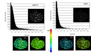
Comparing uFRET (uncorrected for spectral bleed-through - SBT) with PFRET (Processed FRET, corrected for SBT). This PFRET correction software will be available for workshop participants.
