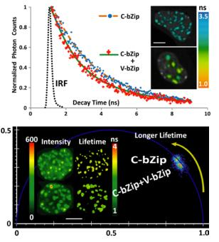
FLIM-FRET Microscopy to investigate proteins dimerizing in the nucleus. Top: Time correlated single photon counting (TCSPC) method (Becker & Hickl). Bottom: Frequency-domain technique (ISS). Nature Protocols 6 (9), 1324-1340, 2011
